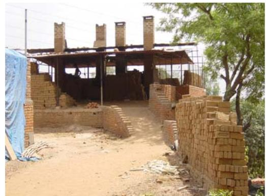
***"I have chosen VSBK for coal savings and more control on plant. With better planning I can fire bricks for 365 days. Now my breakage is reduced to 3-5% compared to 10% in clamp and my coal consumption has reduced to 6 tonnes as compared to 14 tons in clam. I am happy with the plant performance."***
